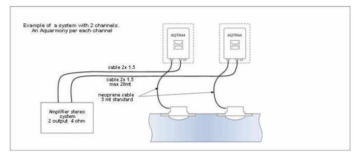
It's very important that the amplifier system has an equalizer and a limiter or compressor in order to protect the loudspeaker form excessive power.
